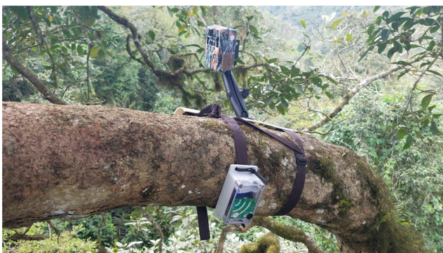
FIGURE 1 Image of a canopy station. The AudioMoth is positioned slightly under the tree to decrease the chance of water buildup and in a weatherproof case that has a membrane to allow sound to pass and a silica packet in the event moisture enters.
